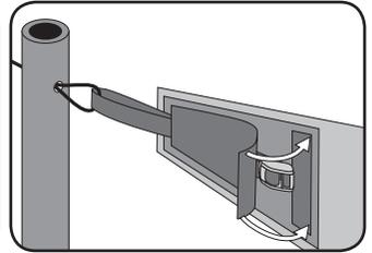
Push the clip and excess webbing back in the pocket and close it using the velcro.
