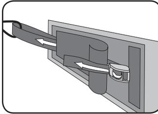
Slide the webbing through the clip to adjust the length of the end straps.
