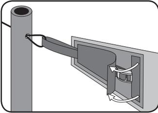
Open up the pocket and pull out the clip and the excess webbing.
